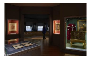
The second gallery contains a darkened, low-ceiling height area reserved for the most light-sensitive items. Here, we added discreet deeprecessed downlights to provide lowkey circulation lighting, and integrated the majority of the lighting into the display cases for localised effect and to protect items from UV exposure.
