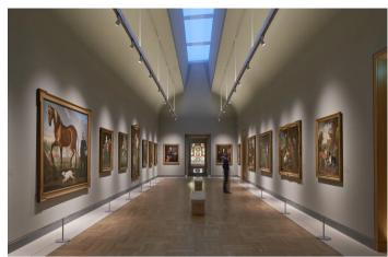
The Long Gallery with its lofty cycloidal barrel vault ceiling is filled with diffuse natural light. We added two custom-made suspended linear profiles that run the length of the space, housing flexible spotlighting to the paintings, as well as uplighting to the ceiling as natural light fades.
